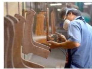
Fig 10.9 Component preparation: spraying chair parts
